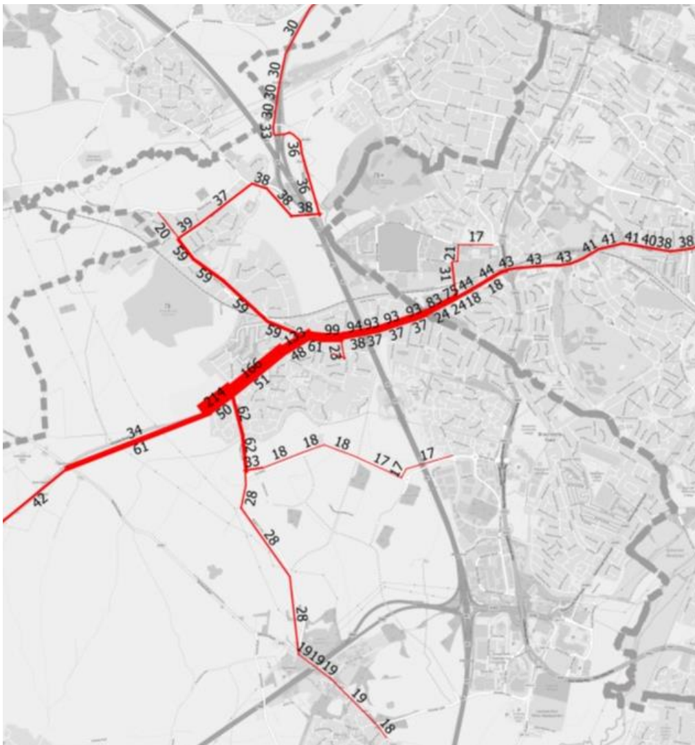
Figure 7-1: AM Peak Distribution of traffic from phase 1 (vehicle volumes based of TRICS mean trip-rate)
